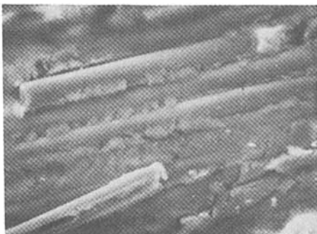
Figure 9. SEM micrographs of the interlaminar fracture surfaces of the composites GD-48, whose matrix is HX-205, and GD-31, whose matrix is F-185.
