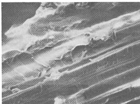
Figure 9. SEM micrographs of the interlaminar fracture surfaces of the composites GD-48, whose matrix is HX-205, and GD-31, whose matrix is F-185.
